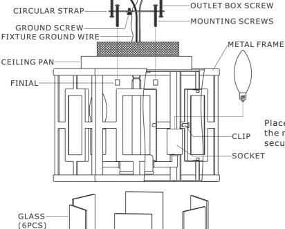
Place the glass inside the metal frame and secure it with the clips.
